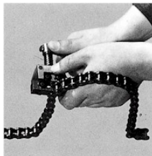
Fig. 4-5 Using the chain breaker
