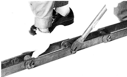
Fig. 11-3 Inserting New T-Pins or Cotter Pins
