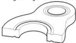
Fig. 2-2 Ring Coining on the Connecting Link
